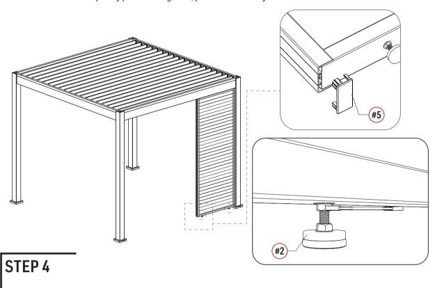
Secure the upper part of the privacy panel to the pergola by using the supplied screws.
