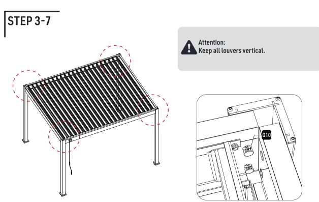
Cover holes in each corner on Beams C/B/B1 with Q10 (plastic cap).
