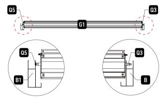
2. Insert **Q3** end of Master Louver **G1** first into 2nd hole of Beam **B**. Then insert opposite side into Beam **B1**.
