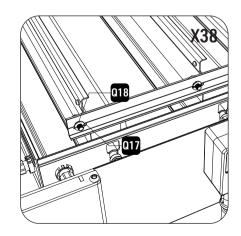
2. Place washer **Q18** onto screw of louver end cap then insert **Q17** into screw of louver end cap. Repeat this with all louver end caps to connect **F** to each louver **G/G1**.
