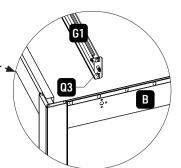
1. Put **G1** (Louvers) in **B**(beam). This is placed in 2nd hole for louver placement, where Beam **B** has opening for **Q8** gear box. **Q8** will install in later step.
