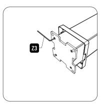
3. Tighten the screw with **Z3** if needed.
