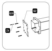
2. Use **Q20**(socket screw 6x35) to install **Q2**(base plate) to attach **A** (post). Use **Z4**(4mm bit ) to secure.
