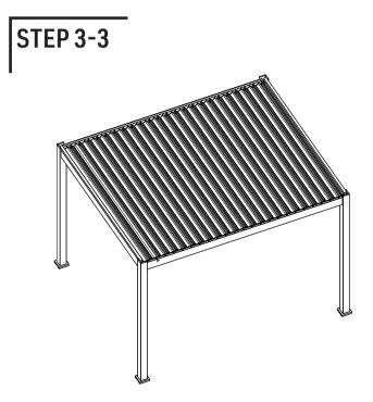
After louvers are installed, lay them in the closed position and insert **Q12** into the opening above spin (**Q6**) on louver end cap.
