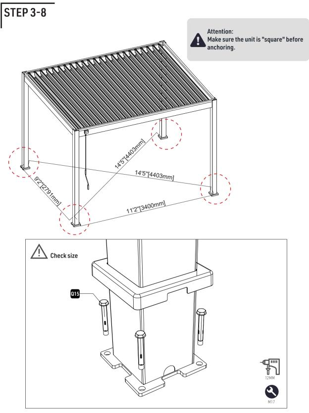
Check all dimensions of the pergola, then anchor base plate **Q2** to concrete foundation using **Q15** (expansion bolt). Caution the post skirting can scratch post.
