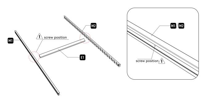
After inserting the E1, please use the screw(W1) to attach the two ends of E1 onto the frame.
