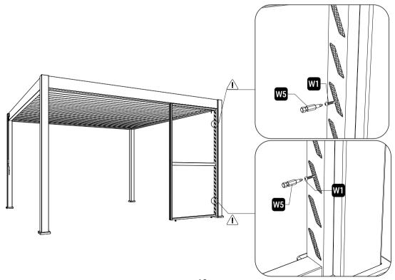
Attach the upper frame of the privacy panel by using screws(W1), then cover the hole with plastic caps(W3).
