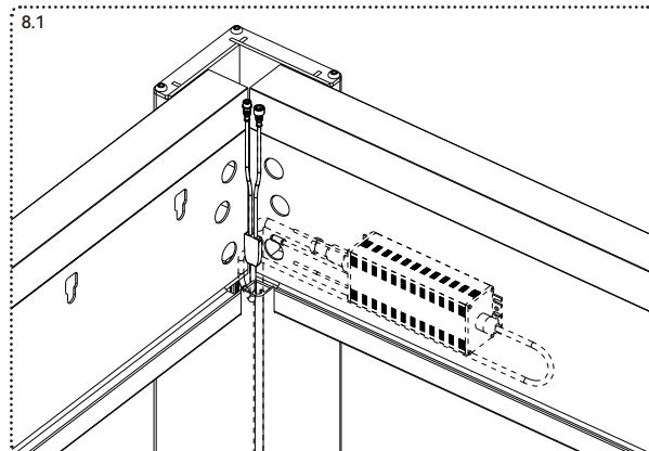
Pull the cable out through the drain outlet and connect it to the transformer.
