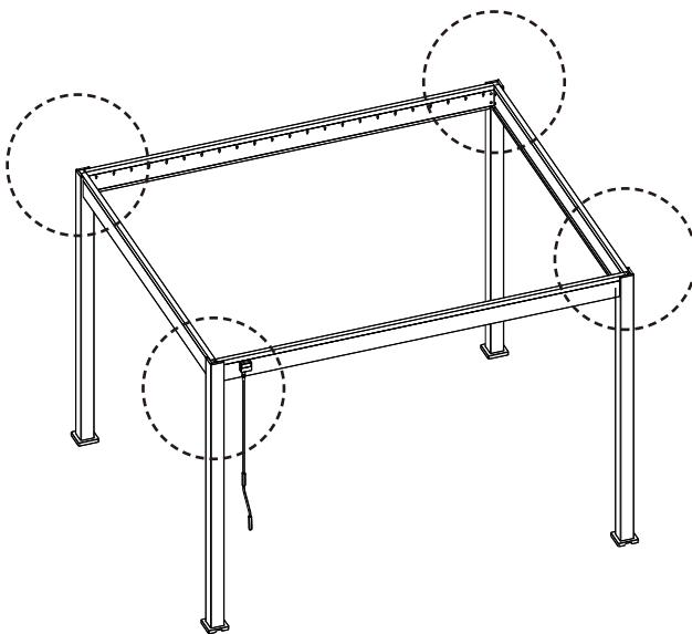
Place the transformer outside and the controller in the cavity of the beam.
