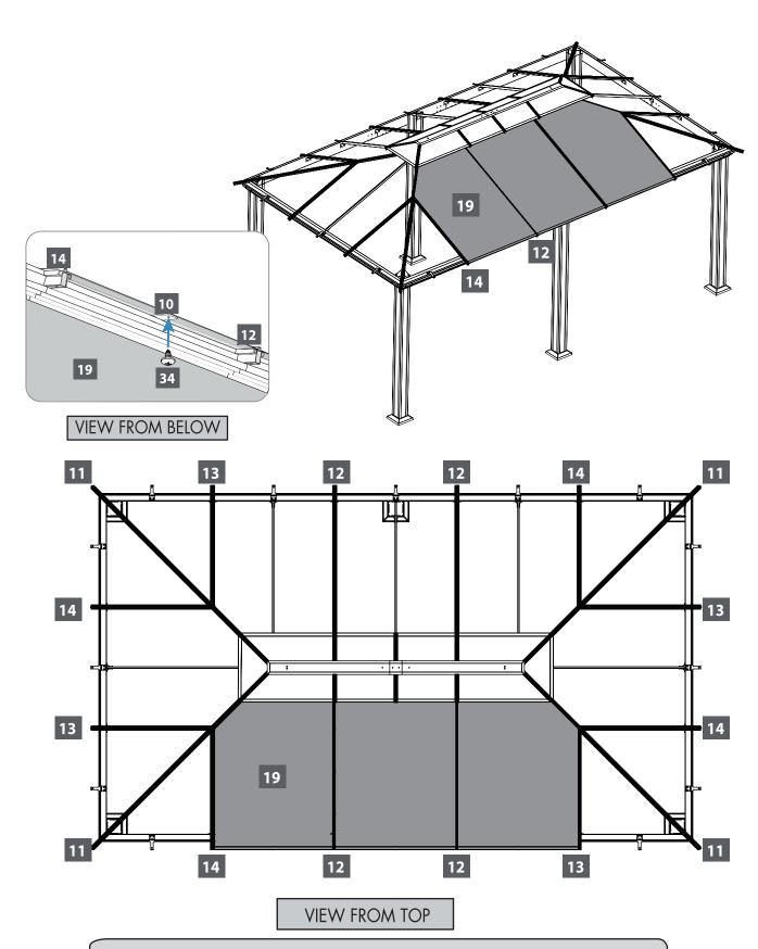
**IMPORTANT:** Make sure that the roof panels are installed exactly in the order shown, otherwise it will be difficult to place the top roof gable profiles.
