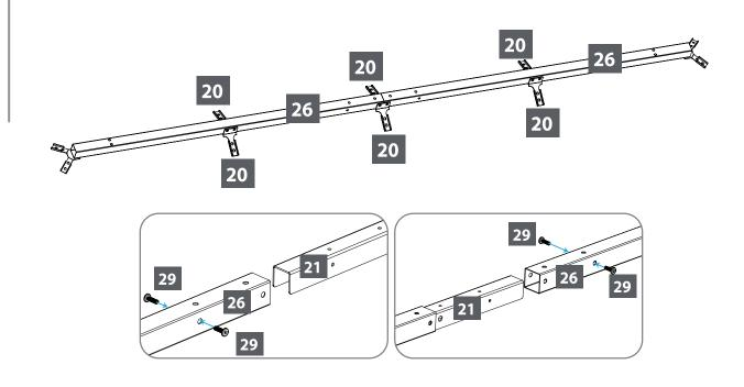
Using screws (45) and nuts (35), connect six top center connectors (20) to roof top connector beams set (26+21+26).
