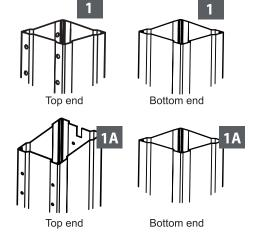
Place corner profiles (1) parallel to each other on the ground. Attach one corner roof connector (4) to each top end as shown and fasten with screws (30).
