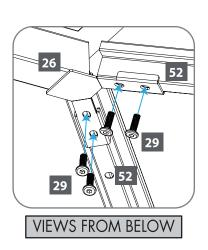
Install roof top connector beam set (26+21+26) to the U-shaped connectors (23) on the lower roof top connector beam set (22+21+22) by screws (33) from below as shown.
