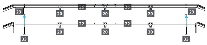
Using screws (29), connect two roof gable profile (53) to top center connectors (20) at the MIDDLE of roof top connector beam (26+21+26).
