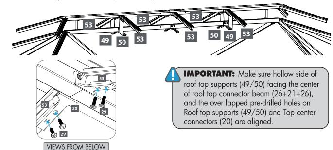
Install roof gable profiles (53) and roof top supports (49/50) to top center connectors (20) at the two end of roof top connector beam (26+21+26) by screws (29) EXACTLY as shown. The screws (29) must go through roof top supports (49/50) and top center connectors (20) than fixed on the roof gable profiles (53).
