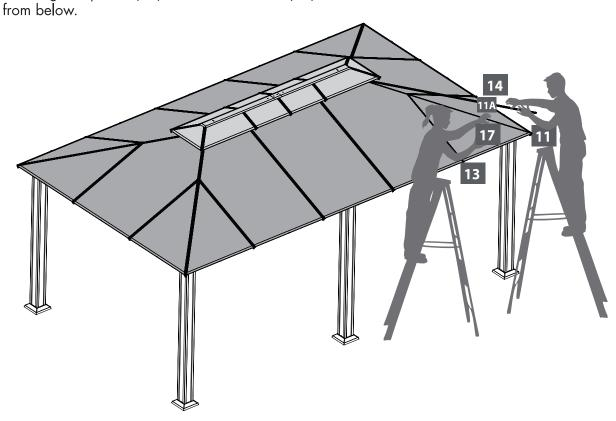
Place the roof gable profile (13A) on top of roof gable profile (13), fasten with screw (32) from below.
