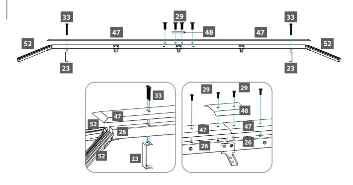
Using screws (29), connect roof gable profiles (52) to roof top connector beam set (26+21+26).
