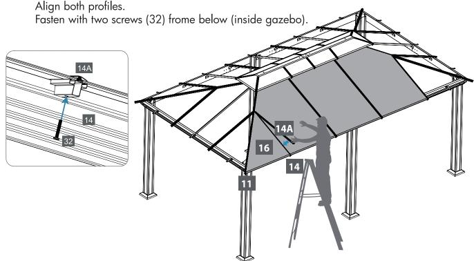
Fit roof panel (15) on top of roof gable profiles (13,14) and fasten with one screws (34) underneath of outer roof connector (10).
