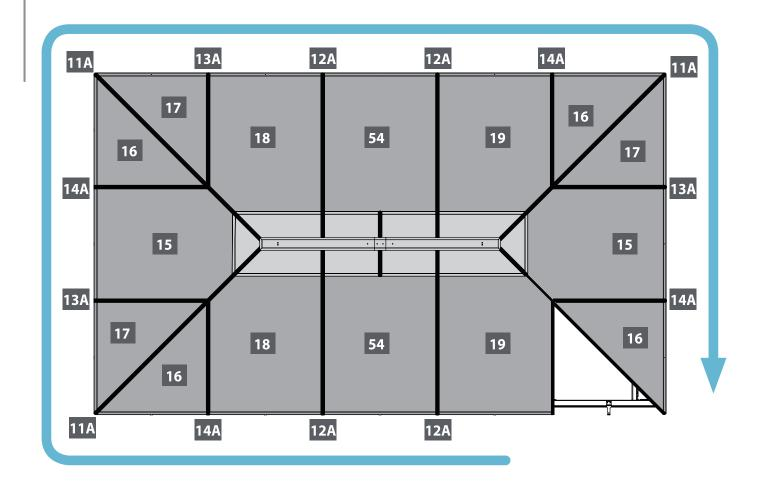
Place the roof panel (16,17) on top of profiles (11,13,14), fasten with screw (34) from below.
