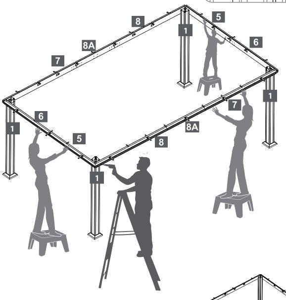
**IMPORTANT:** After this step you should place the gazebo frame in its desired location. Make sure all corners are squared at 90 degrees. Connect middle profile (1A) on middle rail (8A).
