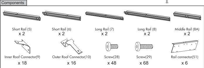
Insert rail connector (51) into blunt end of short rail (5) secured with screws (28).
