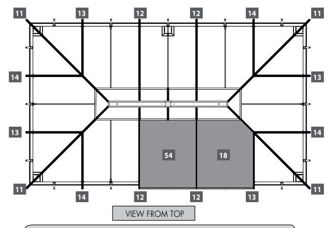
**IMPORTANT:** Make sure that the roof panels are installed exactly in the order shown, otherwise it will be difficult to place the top roof gable profiles.
