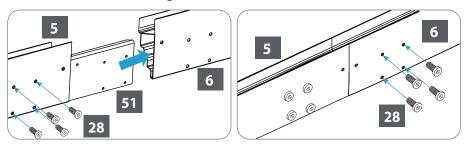
Insert rail connector (51) into blunt end of long rail (7) secured with screws (28).
