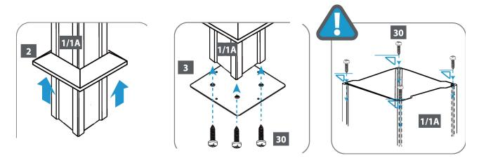
Leave support frames (2) about 10" over lower end of corner profiles (1/1A) until step 4. (Secure the gazebo to the ground)
